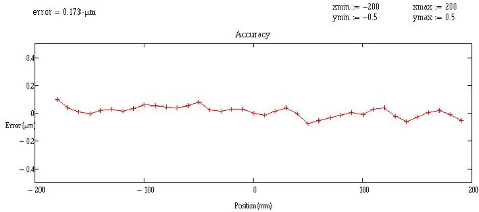
For a combined XY motion, after error compensation, both X and Y-axis error are less than +/-250.
