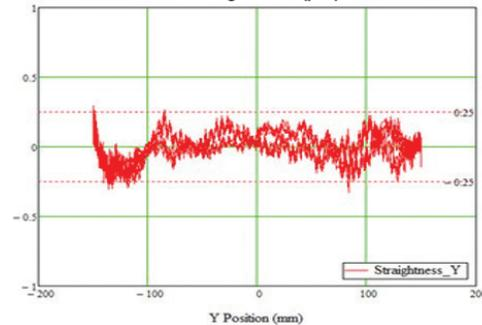
Straightness after mapping within  $\pm 0.25 \mu\text{m}$  @ 1m/s.
