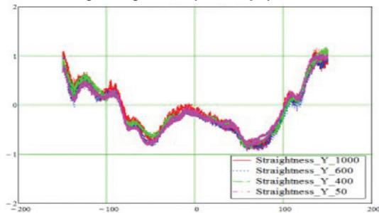
Straightness within  $\pm 1 \mu\text{m}$  @ 1 m/s and repeatability of Straightness within  $\pm 0.25 \mu\text{m}$ , ideal for mapping.
